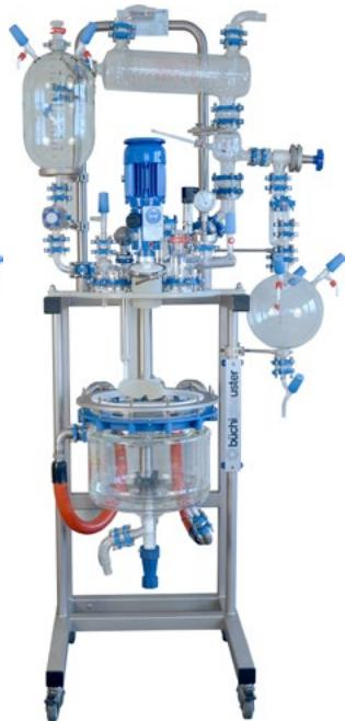
*midiPilot® with multipurpose glass overhead and interchangeable 20 and 30 liter glass vessel
