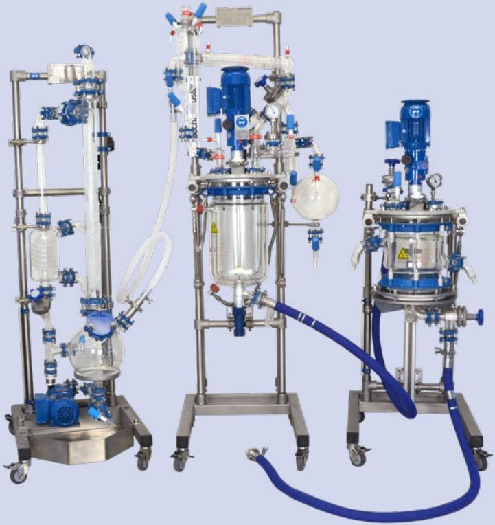
Gas scrubber, miniPilot® reactor, nutsche filter (stirred)
