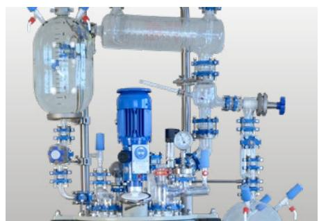
*Multipurpose distillation glass overhead with spiral condenser, reflux divider, phase separator and distillate receiver
