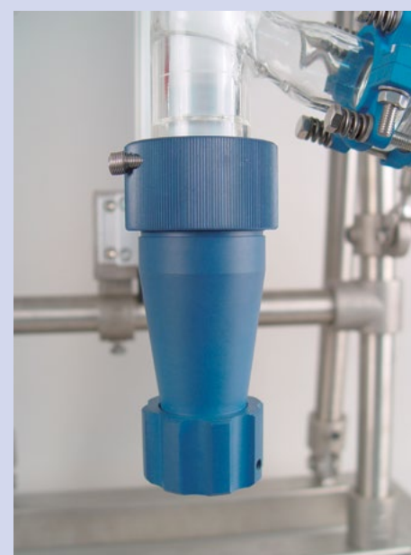
Flush-mount drain valve Totvolumenfreies Bodenventil
